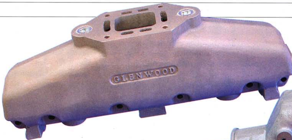
This is a high-quality aftermarket exhaust manifold and elbow made by Glenwood Marine. They are exact replacements for the MerCruiser cast-iron manifold and elbow but are made from aluminum. The weight savings is impressive. It can be purchased either hard-anodized for corrosion protection (shown) or polished.
