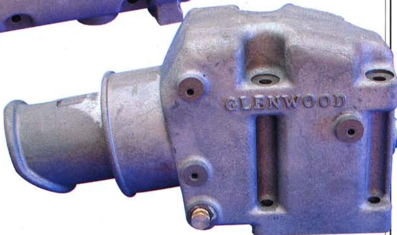
This is a high-quality aftermarket exhaust manifold and elbow made by Glenwood Marine. They are exact replacements for the MerCruiser cast-iron manifold and elbow but are made from aluminum. The weight savings is impressive. It can be purchased either hard-anodized for corrosion protection (shown) or polished.
