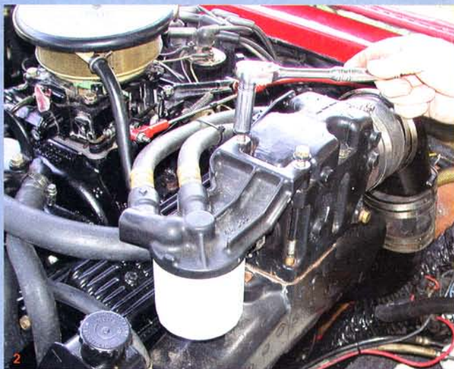
1 Remove the hose clamps that connect the manifolds to the exhaust. 2 In this case, we had to remove the oil filter on the port side.
