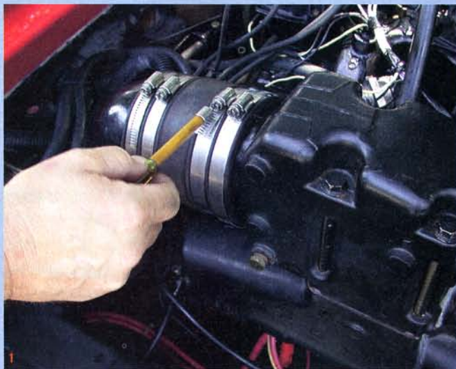
1 Remove the hose clamps that connect the manifolds to the exhaust. 2 In this case, we had to remove the oil filter on the port side.
