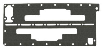
2. Inspect your powerhead, if the cylinder block has water passage O-rings (see A.) the gasket must be modified.
