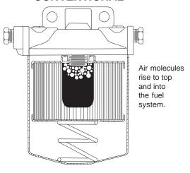
\*For trouble free boating always remember to replace your water/fuel separating filter after every 50 hrs. of engine operation!
