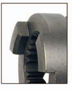
Notice bevel cut and No splines on the lugs.
