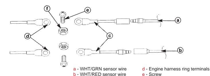
4. Connect WHT/RED and WHT/GRN engine harness wires to the ring terminal adaptor wires
